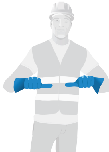
RETRACT HYDRAULIC BOOM OR TROLLEY IN (TOWER CRANE) Both fists in front of body with thumbs pointing towards each other.
