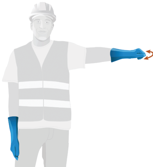
STOP (B) Arm extended, palm down, move hand right and left. Usually for different level operations.
