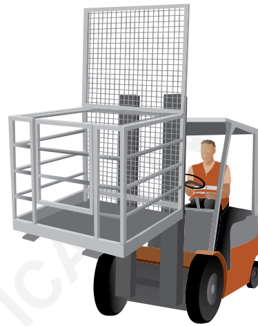
Figure 6: Forklift-lifted work platform.
