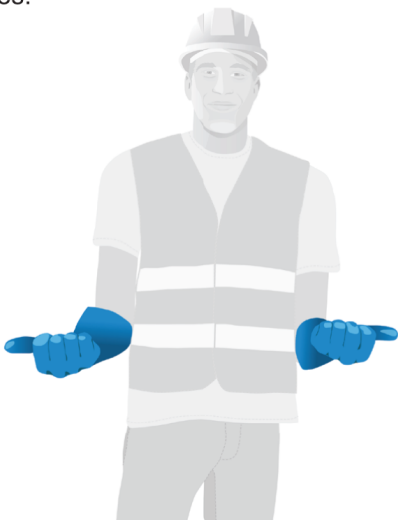
EXTEND HYDRAULIC BOOM OR TROLLEY OUT (TOWER CRANE) Both fists in front of body with thumbs pointing outward.
