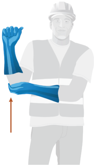
USE FLYLINE (AUXILIARY HOIST) Tap elbow with one hand, then use regular signals.
