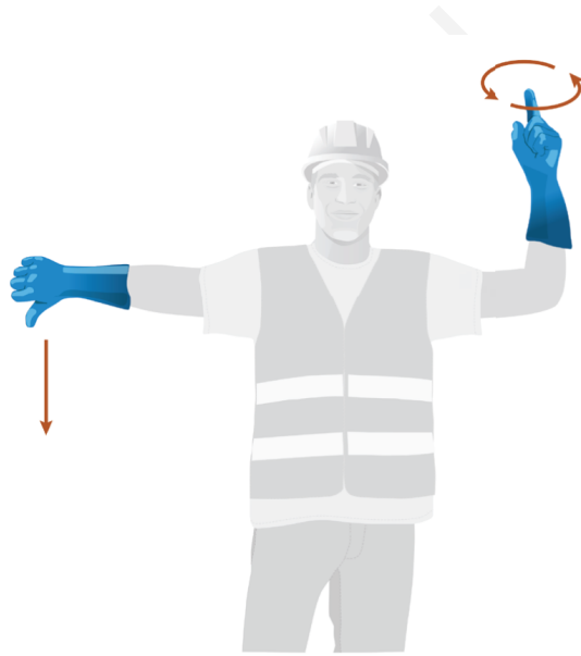
LOWER THE BOOM AND RAISE THE LOAD One arm extended, fingers closed, thumb pointing downward. Other arm vertical with forefinger pointing up, move arm in horizontal circles.
