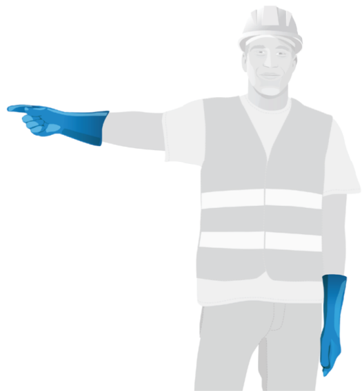
SLEW Arm extended, point with finger in direction of swing of boom.
