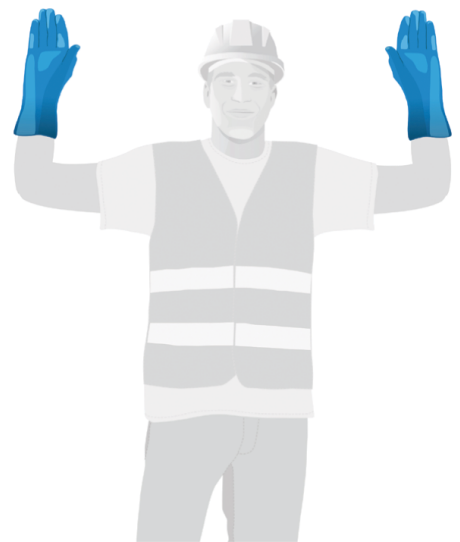
EMERGENCY STOP Extend both arms and hold palms of hands vertical.
