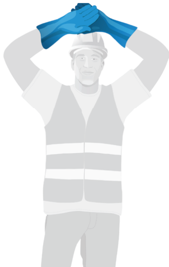
FINISHED WITH CRANE Place arms above head and cross hands.
